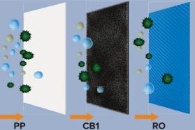
Reduces sediment, rust and suspended particles.
