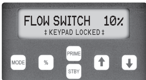
Example of control panel with keypad locked.
