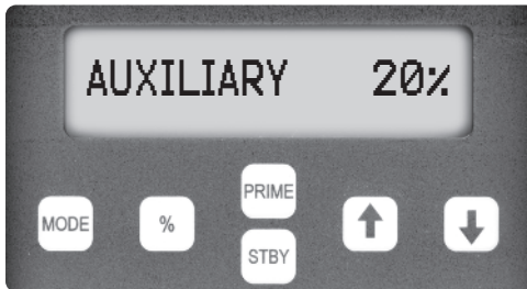
Example of control panel with the pump speed set for 20%.
