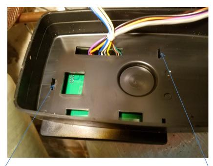
Press in the tabs to remove cover and expose the circuit board.
