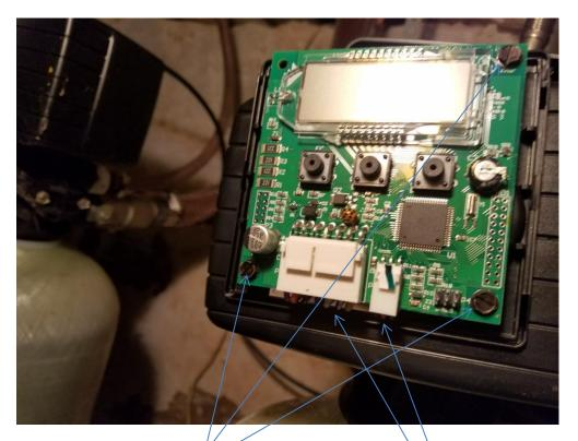
Remove the three screws and gently unplug the wiring.
