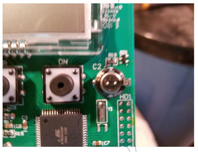
Flip the board over and find the two pins that connect to capacitor.
