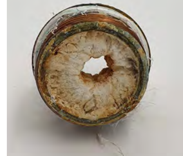
Water flow has slowed because of calcium buildup in pipes
