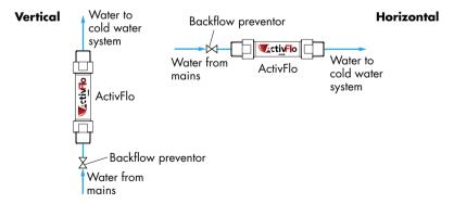
The ActivFlo can be installed vertically or horizontally.
