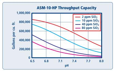
Capacity is based on clean waters that do not contain significant levels of organics, iron, manganese, or other contaminants. The chart is based on 50 ppb of arsenate (As+5) in the feed and TDS less than 500 ppm. ASM-10-HP removes only modest amounts of As+3, therefore pre-oxidation to As+5 may be required. No engineering downgrade has been applied.
