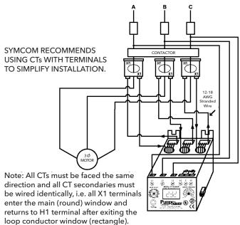
Every CT secondary must make five passes through the corresponding main conductor window on the Model 777-KW/HP.
