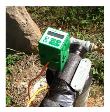
Using the Well Watch for long term monitoring offers many benefits over traditional level meters including the low cost and ease of use. There is also a minimal risk of well contamination since there is no need to lower anything into the well, which makes it a perfect choice for potable, contaminated or caustic wells. The *Sonic Sense* sound waves work equally well at any angle and can even travel around corners in the well casing.
