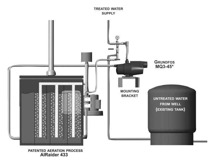
Figure 3 Diagram of Installed System (sold separately)
