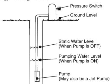
**CAUTION:** If the pumping level used to calculate pipe requirements for a well is substantially above the bottom and the pumping level drops due to drought or other conditions, the pressure rating of the pipe could be exceeded.
