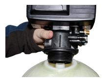
Install the Backwash Control Valve by fitting it onto the top of the tank and that the Riser Tube from the Tank is fitted into the bottom hole of the Control Valve. Twist the Control Valve clockwise onto the top of the Fiberglass Mineral Tank until tightly secured with hand strength.
