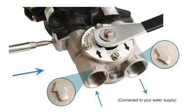
2.) Insert the Control Valve into place with the Bypass and then fasten with the clips. Make sure not to pinch the O-ring that are on the valve ports. Turn handle so it's pointing toward bypass.
