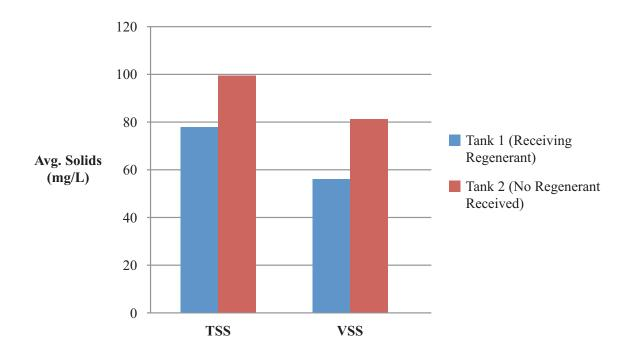
The addition of regeneration wastes that contain large concentrations of excess sodium can, however, be detrimental to solids settling and, therefore, produce a lower quality effluent. Such higher concentrations can be from the operation of a softener in an inefficient manner (</= 1000 gr/lb) in relation to the excessive use of salt for the removal of hardness.
