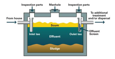
**Figure 3.** Typical one compartment septic tank illustrating solids separation and development of clear zone. The outlet tee (on right) is designed to draw clarified effluent from the clear zone, through an effluent screen, and then out of the tank, and convey it to the next component (NFSC 2000).
