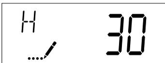
5. Press the Extra Cycle button. Use this display to adjust the Fixed Reserve Capacity. This option setting is
