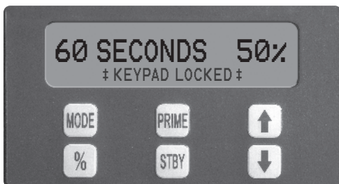
Example of control panel with keypad locked.
